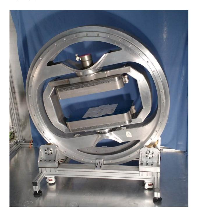
A prototype 'mini' MRI scanner, developed by Imperial College London, that could be used for diagnosing knee injuries. Credit: Imperial College London
