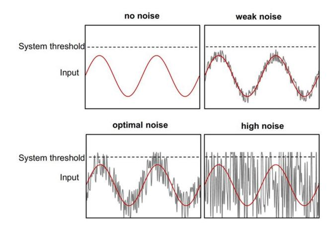
Stochastic resonance occurs when an optimal level of noise is added to a weak signal. In this example the signal alone (red line) remains below the threshold for detecting the signal (dotted line). Adding an optimal amount of noise raises the stimulus periodically above the system threshold. If the added noise is too weak, the threshold is not crossed. Conversely, if the noise is too strong, the signal remains buried and cannot be discriminated from the noise. Author provided
