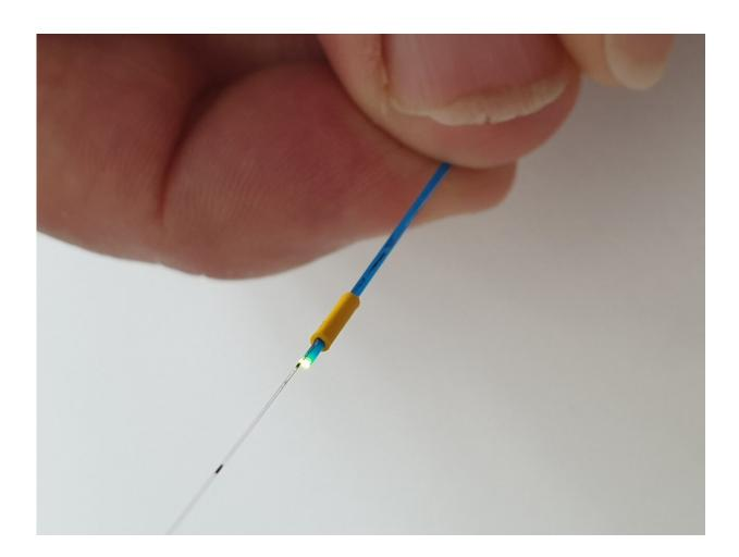
The new device can measure continuous and instantaneous blood flow using optical heating at a low power input with an LED light source. Credit: Flinders University
