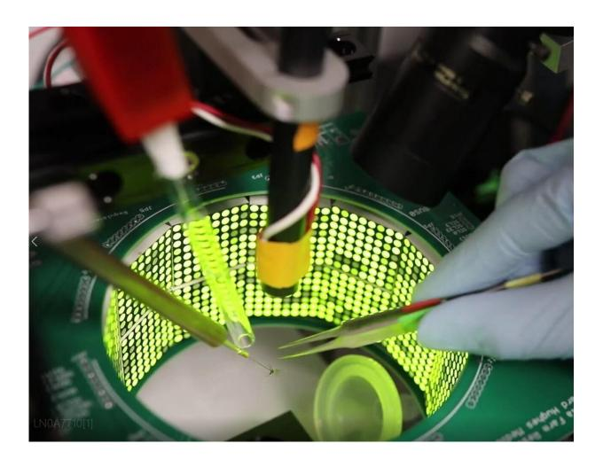
Top-view image of the arena, or flight simulator, used to present different visual objects and olfactory cues to tethered mosquitoes. Credit: Kiley Riffell
