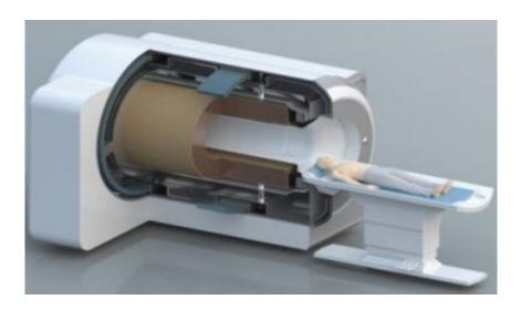
MRI transmits a high frequency magnetic field of thousands of hertz to the human body, and displays the image signals generated from atomic nuclei in the body in a 2D or 3D cross-sectional image. Credit: Korea Electrotechnology Research Institute (KERI)
