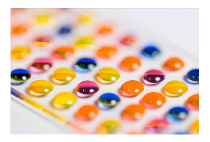
Array of microdroplets with various reactants on the chemBIOS chip-based synthesis platform. Credit: Maximilian Benz, KIT
