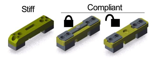
Computer models of fixation plates for mechanical load transfer. Credit: Joel Boerckel
