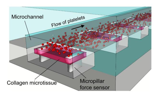
This diagram demonstrates how the engineered tissue model works to mimic the clotting upon blood vessel injury. Platelets adhere to the collagen microtissue that represents the collagen layer in the blood vessel. The micropillars that support the microtissue sense the stiffness of the microclots that form when exposed to different flow rates, which mimic venous or arterial flow in the body. Credit: Zhao, Neelamegham, et al/*Nature Communications*
