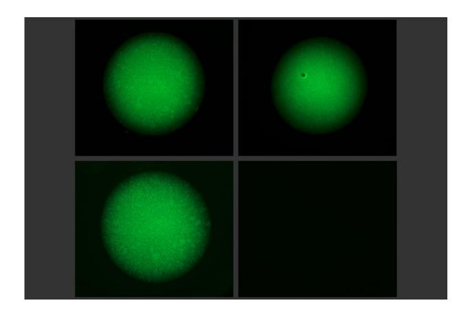
MIT engineers created a DNA-acrylamide gel that can be degraded by DNA-editing enzymes. At right, the gel is broken down after two hours of exposure to a DNA "trigger sequence." At left, the gel is exposed to DNA that doesn't contain the trigger sequence, so it remains intact. Credit: James Collins
