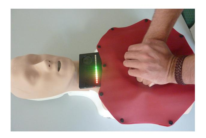
Illuminated LEDs at the upper edge of the mat indicate whether the first responder is administrating chest compressions correctly. Credit: © Fraunhofer ISC
