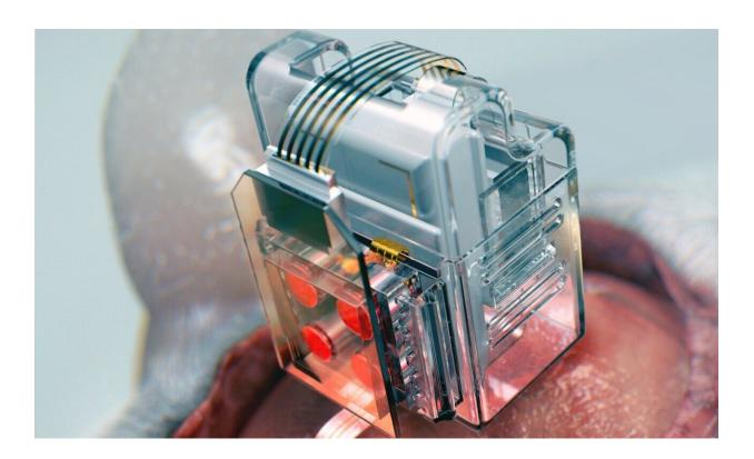
The device, using Lego-like replaceable drug cartridges and powerful bluetooth low-energy, can target specific neurons of interest using drug and light for prolonged periods. Credit: Korea Advanced Institute of Science and Technology
