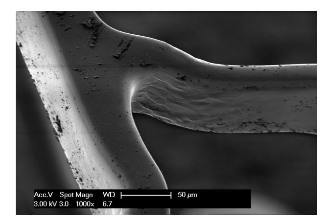
The coating is barely changed after 30 days of exposure to the test fluid. Credit: Fraunhofer IKTS
