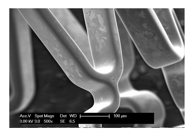
A stent coated with titanium oxynitride. Credit: Fraunhofer IKTS
