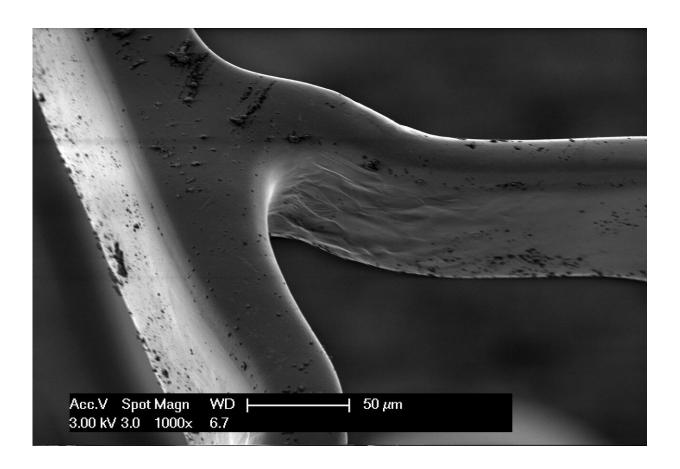
The coating is barely changed after 30 days of exposure to the test fluid. Credit: Fraunhofer IKTS
