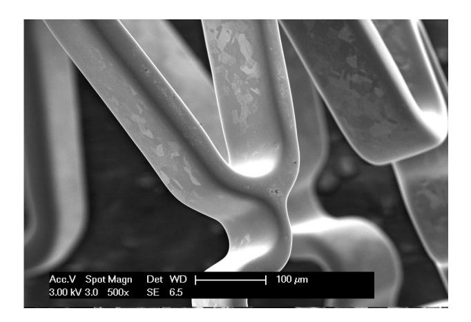
A stent coated with titanium oxynitride. Credit: Fraunhofer IKTS
