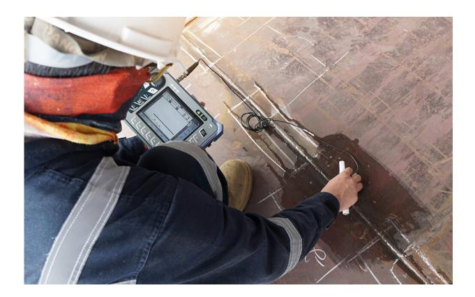
In addition to medical diagnostics, ultrasound can be used for many other things, such as examining welded seams in steel piping, as well as testing of different materials used in the oil and gas industry. Credit: NTB Scanpix
