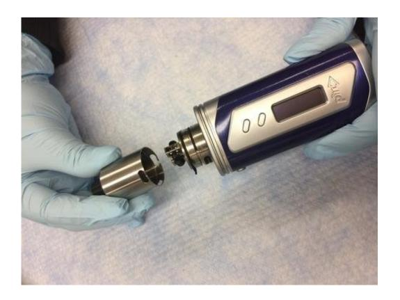
Photo shows a typical tank-style electronic cigarette. With the lid off, the atomizer attached to the tank is revealed. Credit: UCR/I. Pittalwala
