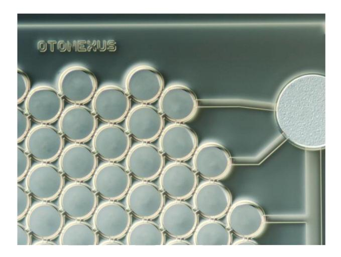
At the heart of the revolutionary otoscope from U.S. company OtoNexus Medical Technologies is a unique CMUT chip from Fraunhofer IPMS based on ultrasound technology. Credit: Fraunhofer IPMS
