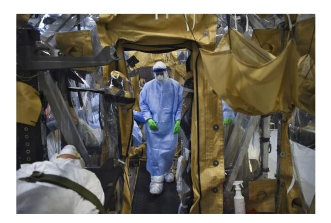
An airman performs the final set of checks during transportation isolation system (TIS) training while practicing patient care in a containment unit. Engineered and implemented after the 2014 Ebola virus outbreak, the TIS is an enclosure the U.S. Defense Department can use to safely transport patients with highly contagious diseases. Credit: Senior Airman Cody R. Miller/U.S. Air Force
