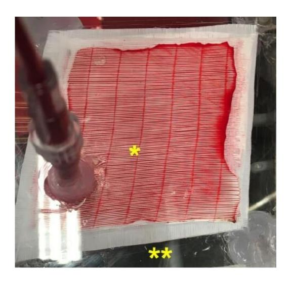
The carbon monoxide photo-remover consists of sealed compartments for blood and gas. Credit: L. Zazzeron et al., Science Translational Medicine (2019)
