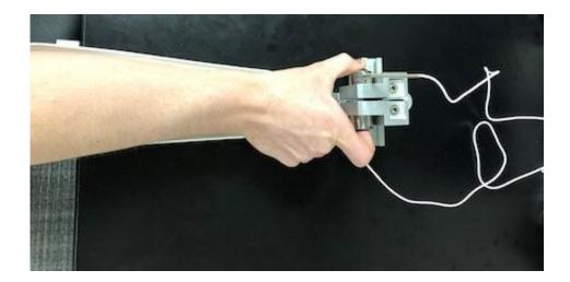
The custom-made arm brace and load cells for precision grip testing. Participants pressed with their thumb and forefinger against two precision load cells while viewing two horizontal bars displayed vertically on the screen. Credit: McKinney et al
