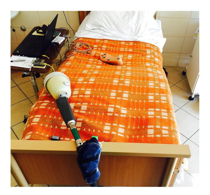
The neuroprosthesis used by a volunteer. The rubber foot is used to test the capability of patients to understand the positions of touch sensations. Credit: Stanisa Raspopovic
