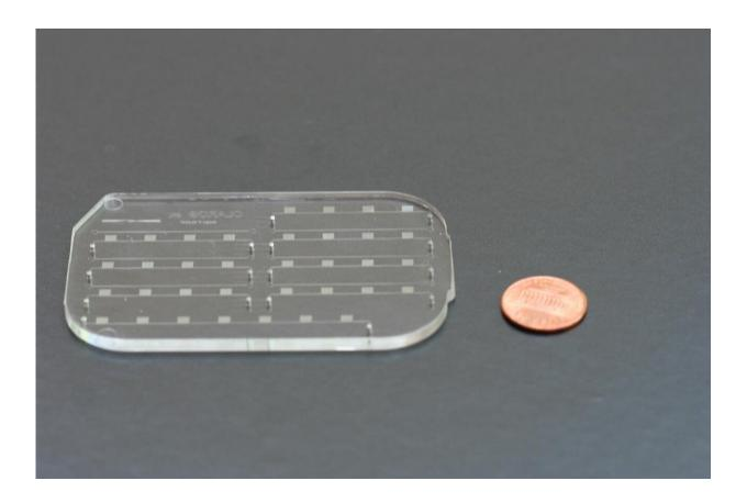
A microfluidic chip used to test for Lyme disease. Credit: Sia Lab/Columbia Engineering and OPKO Health
