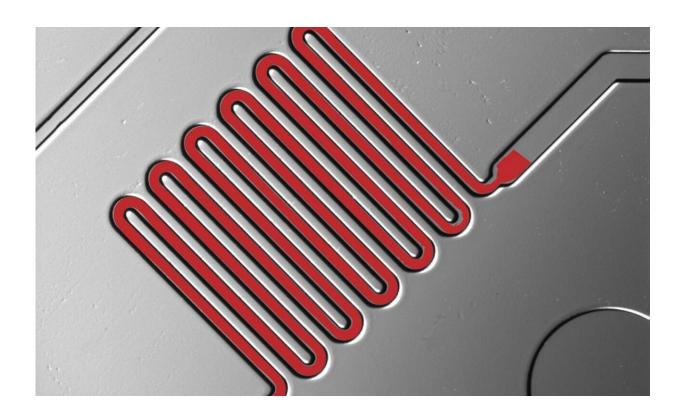
A zoomed photo of fluid moving through a small channel in the microfluidic chip. Credit: Sia Lab/Columbia Engineering and OPKO Health
