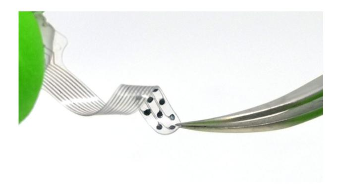
The highly elastic implant conforms neatly to the curved surface of the auditory brainstem and can therefore send highly targeted electrical signals. Credit: EPFL
