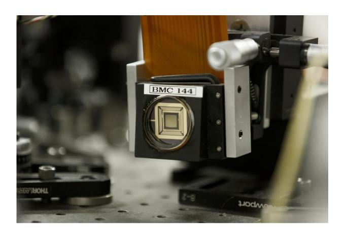
The ophthalmic laser microscope used to collect the first undistorted images of the eye's trabecular meshwork. The equipment includes a deformable mirror able to automatically correct for imperfections in the eye. Credit: James Brosher, Indiana University.
