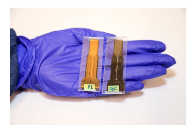
A side-by-side look at platinum (left) and glassy carbon (right) thin-film electrodes for deep brain stimulation. Credit: SDSU
