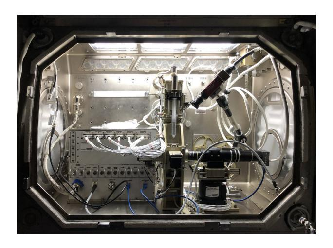
The Ring-Sheared Drop experiment hardware, installed inside the Microgravity Science Glovebox, will help investigators understand protein aggregation associated with devastating neurodegenerative diseases such as Alzheimer's and Parkinson's. Credit: NASA/Kevin Depew
