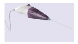
Prototype Raman 'smart needle' probe. Credit: University of Exeter
