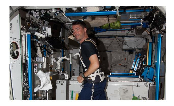
NASA astronaut Reid Wiseman, Expedition 40 flight engineer, equipped with a bungee harness, exercises on the Combined Operational Load Bearing External Resistance Treadmill (COLBERT) in the Tranquility node of the International Space Station. Credit: NASA
