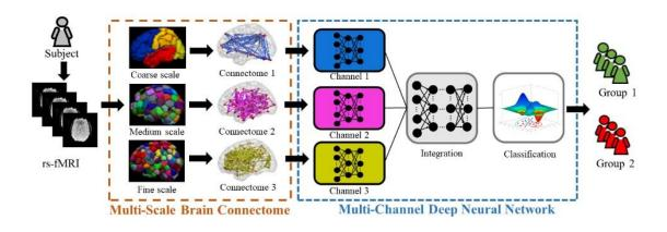
Schematic diagram of the proposed multichannel deep neural network model analyzing multiscale functional brain connectome for a classification task. rsfMRI = resting-state functional MRI. Credit: Radiological Society of North America
