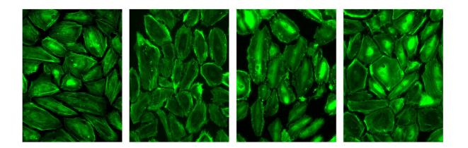
AAV-pulmonary-chip Fig2a - When human endothelial lung cells in the Lung Chip (panel 1) are subjected to strain in the horizontal direction, they reorient themselves vertically (panels 2 and 3), contributing to the leakage of fluid into the air channel. Delivering the AAV gene therapy construct reduced the cells' realignment (panel 4), helping to reduce leakage. Credit: Wyss Institute at Harvard University
