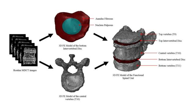
Schematic workflow illustrating methodology from acquisition of images to finite element (FE) modelling of the functional spinal units (FSUs). Credit: SUTD
