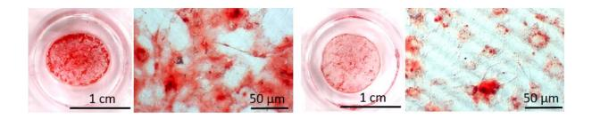
The shape-memory polymer actuator sheet coated with stem cells shrunken when cold (left) and stretched when heated (right). Credit: Polymeric sheet actuators with programmable bioinstructivity, Zijun Deng, Weiwei Wang, Xun Xu, Oliver Gould, Karl Kratz, Nan Ma, and Andreas Lendlein, *Proceedings of the National Academy of Sciences*, 2020, doi: 10.1073/pnas.1910668117
