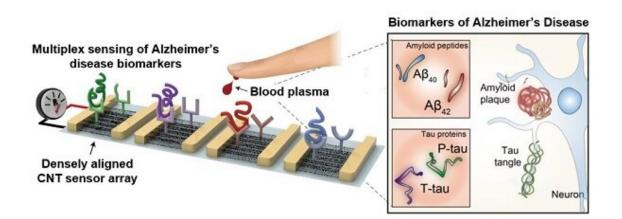
Figure: A schematic diagram of a high-density aligned carbon nanotube-based resistive sensor that distinguishes patients with Alzheimer's Disease by measuring the concentration of four biomarkers in the blood. Credit: The Korea Advanced Institute of Science and Technology (KAIST)
