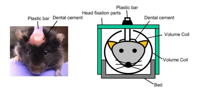
Head immobilization apparatus for conducting awake fMRI scans. Credit: Kobe University
