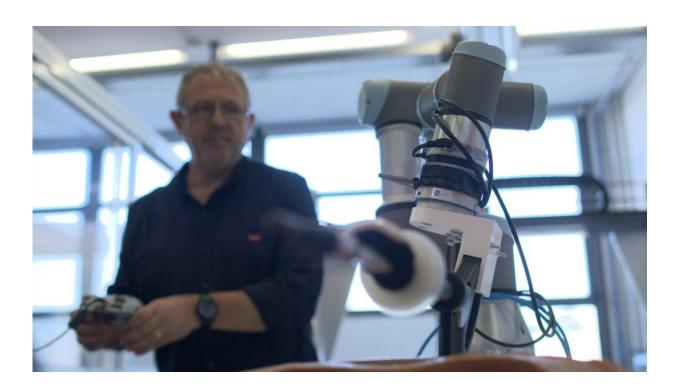
The system will allow for a robotic arm to control the handler that the second doctor currently holds for hours to control the position of the uterus. Credit: UPV
