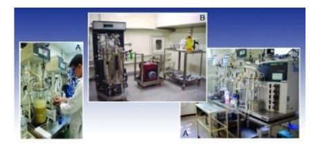
Bioreactors for bench-scale production (A); bioreactor for pilot-scale production (B). Credit: Butantan Institute
