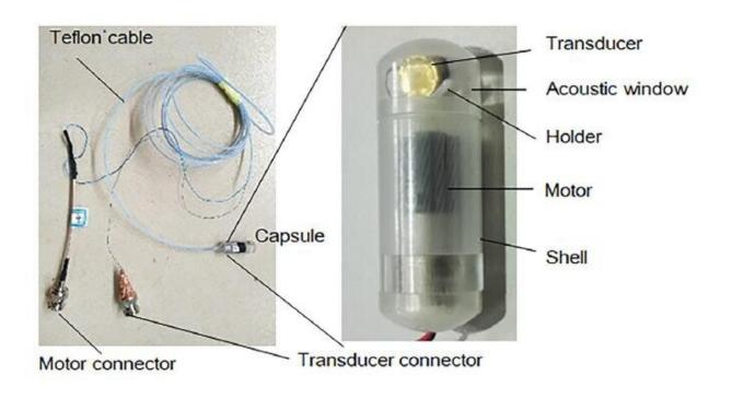
Fig. 1. The final  $\mu$ USCE device. Credit: QIU Weibao
