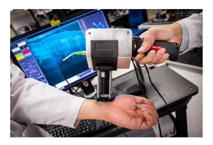
The prototype handheld medical imaging device developed by NTU Assoc Prof Liu Linbo can produce high-resolution images in real-time, and was also designed to be used by medical professionals who do not specialise in imaging or pathology, allowing them to scan patients using the new device in community clinics or at the bedside. Credit: Nanyang Technological University
