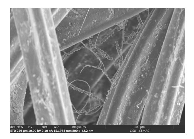
Fungal growth (mold) on nylon carpet fibers loaded with house dust at elevated relative humidity. The image was collected after a 2 week incubation period at 95% relative humidity and 25°C and was viewed with Scanning Electron Microscopy (SEM). Credit: Nick Nastasi
