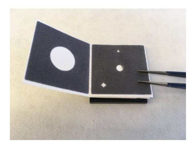
The paper device is folded and unfolded in steps to filter the nucleic acids of pathogens from wastewater samples, then a biochemical reaction with preloaded reagents detects whether the nucleic acid of SARS-CoV-2 infection is present. Results are visible to the naked eye: a green circle indicating positive and a blue circle negative Credit: Cranfield University
