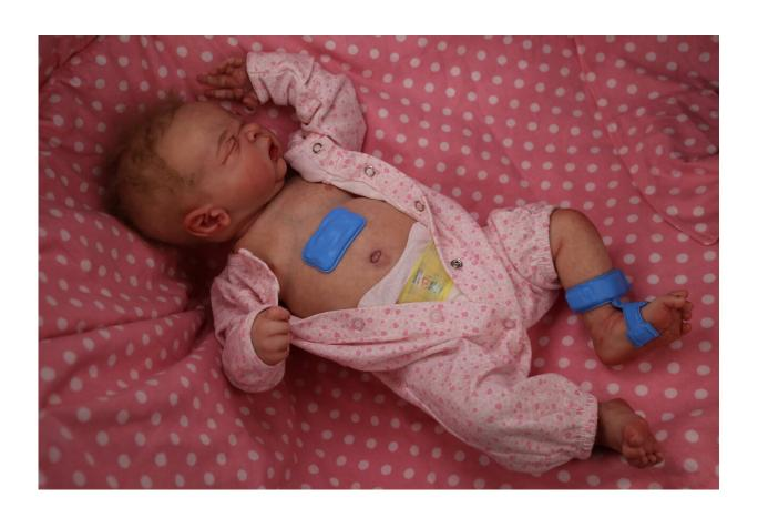
The wireless sensors (in blue) displayed on a model neonate in the lab. Credit: Northwestern University
