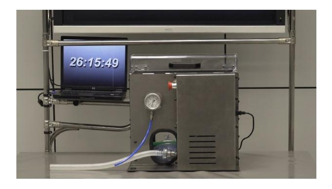
A mechanical ventilator being developed by Spanish automobile manufacturer SEAT at the company's Martorell factory using a windscreen wiper motor
