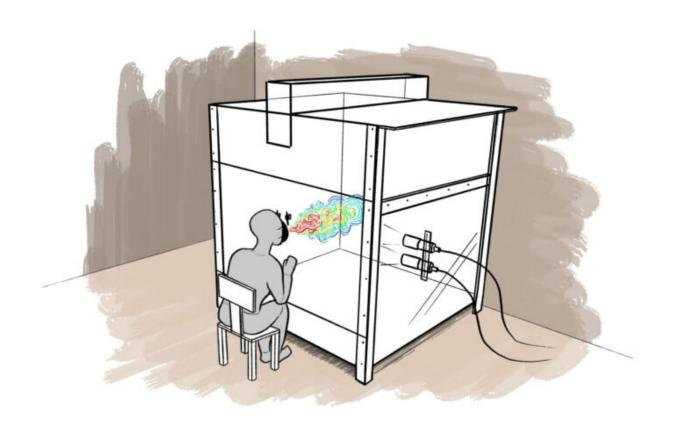
Western Engineering's cough chamber is a two-metre enclosed cube with an opening and chin rest in the front, which is used as an access point for study participants to cough. Within the cube, a camera and a laser are used to determine the velocity of the expelled droplets from the cough. Credit: Frank Neufeld
