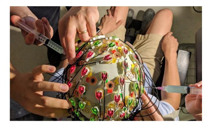
Researchers prepare a test subject by dispensing conductive electrode gel into the electrodes in an EEG cap. Credit: Drexel University
