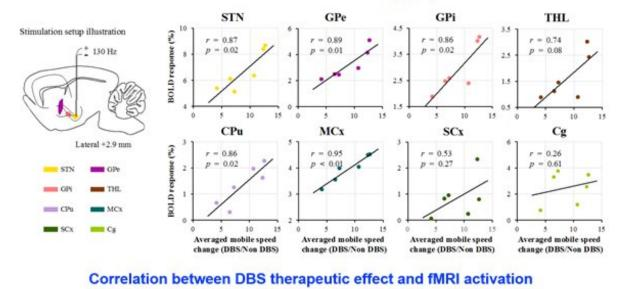
Simultaneous DBS-fMRI using graphene fiber electrode in Parkinsonian rats revealed close relationship between fMRI activation and DBS therapeutic effects. Credit: College of Engineering, Peking University
