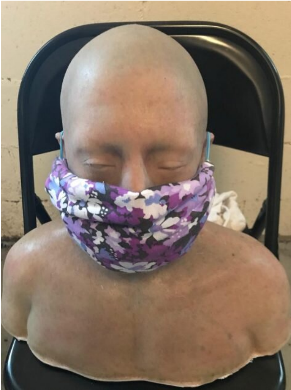
One of three homemade face coverings tested out by the researchers. The silicone headform was a donation from Joshua Turi. Credit: Beizhan Yan
