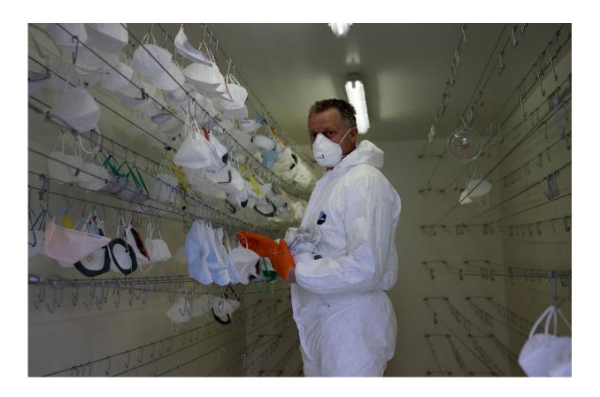
A worker at the ECCA laboratories hangs mouth masks in the Clean Mask Decontaminating Room in Merelbeke, Belgium, Tuesday, April 28, 2020. The converted shipping container holds 1500 masks and runs on a six hour disinfection cycle with a hydrogen peroxide dry mist. With mouth masks in short supply for healthcare workers in Belgium against coronavirus (COVID-19), innovative solutions have been made to deal with the crisis. (AP Photo/Virginia Mayo)
