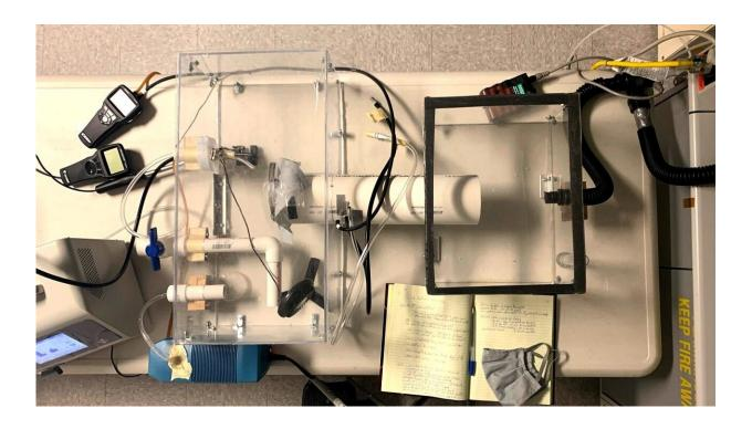
The experimental setup for the mask test. Different combinations of cloths are placed over the pipe, a fan blows particles at the fabric, and researchers check how many particles made it through the second box. Credit: Supratik Guha
