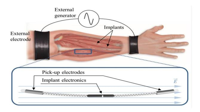
The method of wireless energy transfer via volume conduction consists of using the body's own tissues as a channel for transferring electrical power. The authors propose delivering currents with magnitudes above one ampere that are harmless due to their high frequency. Credit: BERG-UPF
