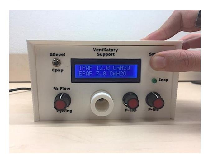
Display panel for the low-cost, easy to build prototype ventilator, which could be used to support COVID-19 treatment in low income regions or where ventilator supplies are limited. Credit: Prof. Ramon Farré.
