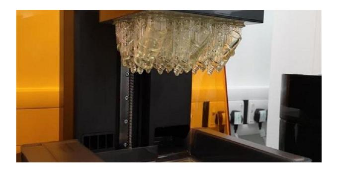
The valves being manufactured in a 3D printing machine at the University of Leeds. Credit: University of Leeds
