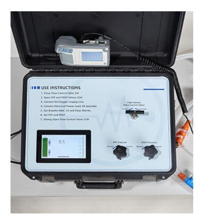
The Novel Emergency Response Ventilator (NERVe) design incorporates components that are not normally used in ventilator manufacture, to avoid disrupting supply chains for ventilator parts. It is designed to meet the functional requirements of COVID-19 patients requiring mechanical ventilation but will need to be approved by the U.S. Food and Drug Administration before it can be used with patients. Credit: Lawrence Livermore National Laboratory
